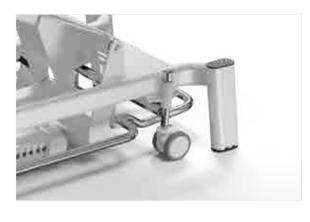
The lift able Stand-by Castor System adopts the medical castors and the connecting rod operating system. The four castors can be released and retracted synchronously by foot pedal control. The bed can be moved easily when wheels are released, and the stability of the bed will be increased when the castors are folded up. Castor system must be installed by the original factory. Users are not allowed to install the castor system without permission to avoid accidental injury.
